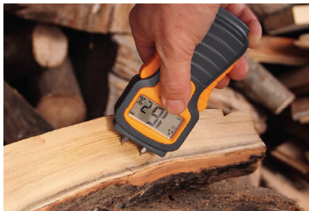
Figure 1: Example of a rapid moisture meter with electrodes (prongs)
