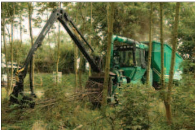
Figure 3: The Silvatec chipper is a purpose-built machine including a chipper and a collection container.
