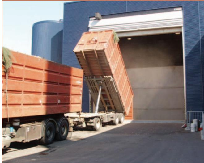
▲ Chip delivery to a reception pit inside a building - note the height of the gate.
