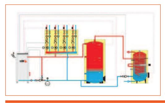
Figure 2: Schematic of a Fröling domestic gasifying system.<sup>1</sup>
