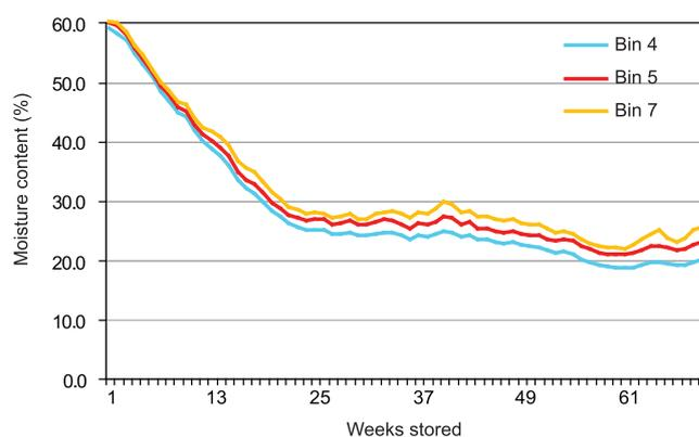
Figure 5: Drying rates of bin 4 (covered sides and top), 5 (covered top) and 7 (uncovered) decreasing with less cover of stacks.
