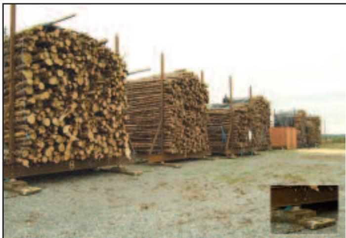
Figure 2: View of the bin trial in September 2007. Bin 1 is ready to be refilled. Note the load cells under the bins (also see insert).
