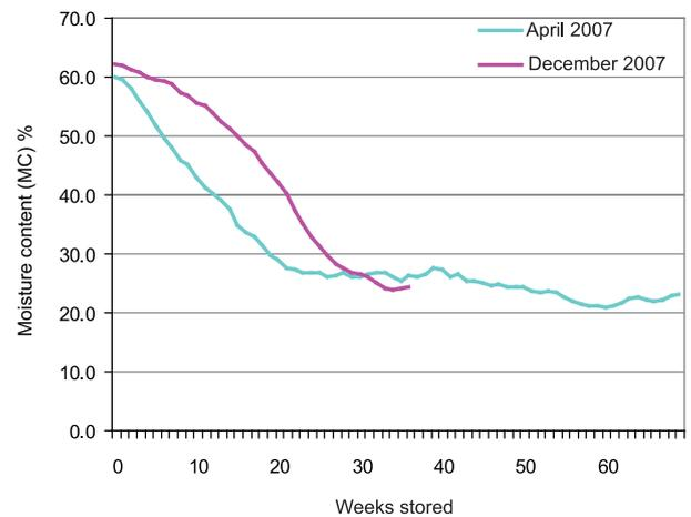
Figure 4: Time required for drying to 30% moisture content, relative to the start month of the storage trial.
