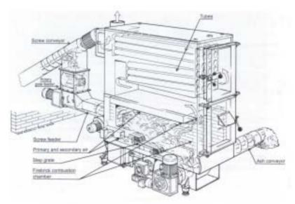
*Figure 6: Automatic Wood Chip-fired Heating System* Source: Centre for Biomass Technology (1999). Used with permission. Drawing by Maskinfabrikken Reka A/S.
