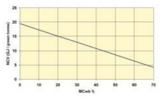
Figure 2: Net Calorific Value of Wet Wood (Based on equation in Centre for Biomass Technology, 1999.).
