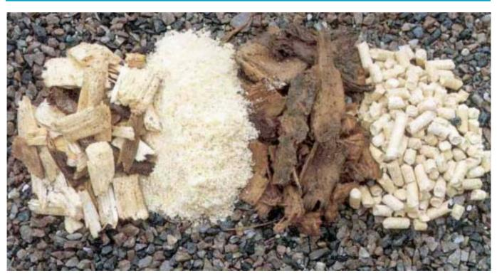
*Figure 5: Forms of Wood Fuel Forest wood chips, sawdust, bark, wood pellets* Source: Centre for Biomass Technology (1999). Used with permission. Photograph by Flemming Rune, Danish Forest and Landscape Research Institute (FSL). easier to handle. Some countries have well established quality standards for firewood, wood chips and wood pellets. Other countries do not. There is work progressing at EU level to develop common standards for solid biofuels.
