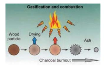
*Figure 3: How a Wood Particle Burns* Source: Centre for Biomass Technology (1999). Used with permission.
